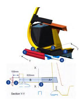
Figure 7.2.6.4 SEM1 Body structure rear zone (See Appendix 4 for larger image)
