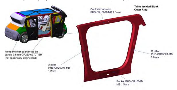
Figure 7.2.5.20 SEM1 outer ring and approach for A surfaces (See Appendix 4 for larger image)
