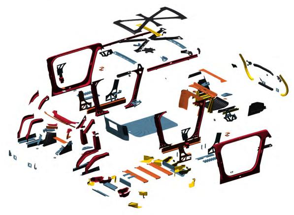
Figure 7.2.1.4 Steel E-Motive SEM1 BIW AHSS grades (exploded view) (See Appendix 4 for larger image)
