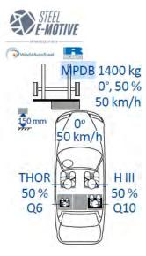
Figure 4.2.4.1 EuroNCAP Moving Progressive Deformable Barrier (MPDB) test protocol
