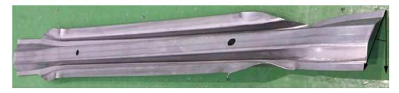
Figure 5.9: A roll stamped door part formed on a conventional roll forming line eliminates the need for welding brackets at the edges.
