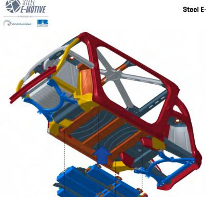
Figure 7.3.1.2 Steel E-Motive battery assembly into body structure
