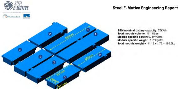
Figure 6.2.1.3 SEM1 battery module sizing and specifications
