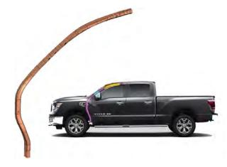
Figure 5.11: 2016 Nissan Titan XD: Door-To-Roof Support.
