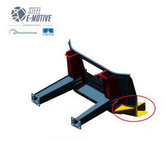
2 part FRONT TORQUE BOX (INNER & OUTER) 1.0mm CR8501180T-DH
