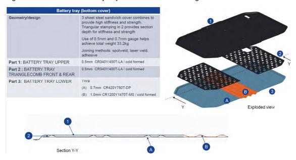
Figure 7.3.3.1 Battery tray design and AHSS grades (See Appendix 4 for larger image)
