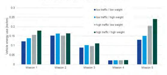
Figure 9.3.2.5.7 SEM1 predicted vehicle energy consumption for Brighton and Hove city mission profiles (values without autonomous vehicle cycle smoothing)
