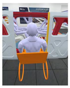
Figure 7.1.4.1 SEM1 wheelchair user vehicle access evaluation using Virtual Reality tools
