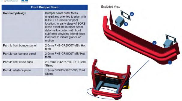
Figure 7.2.3.14 Front bumper beam AHSS grades (See Appendix 4 for larger image)
