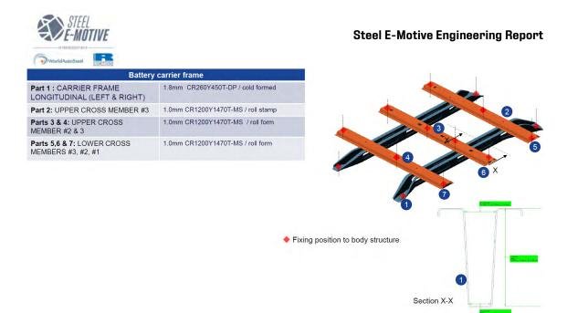
Figure 7.3.2.1 SEM1 battery carrier frame design and AHSS grades (See Appendix 4 for larger image)
