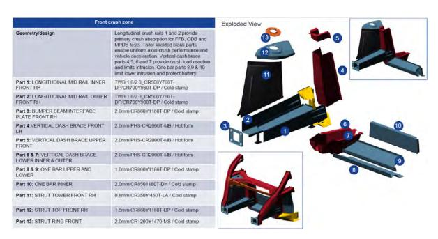
Figure 7.2.3.15 Front crush zone AHSS grades (See Appendix 4 for larger image)
