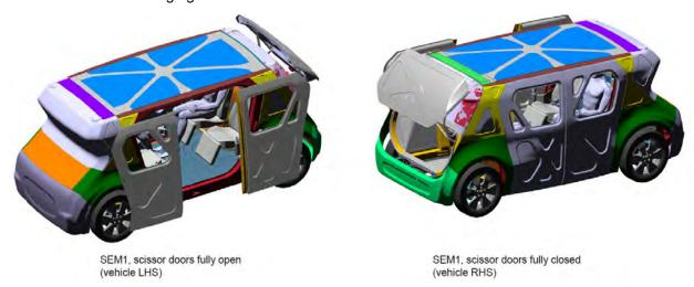
Figure 7.4.1.2.1 SEM1 scissor doors – open and closed positions
