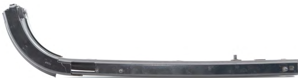
Figure 6.3.5.1.2 Ford B-Max sliding door track profile (plan view, image from a2mac1)
