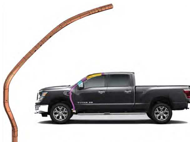
Figure 5.11: 2016 Nissan Titan XD: Door-To-Roof Support.
