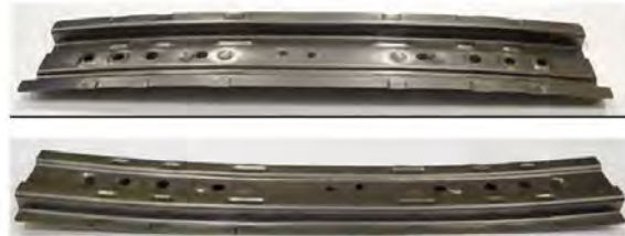
Figure 5.10: Center roof reinforcement adopted with use of 1470MPa grade cold-rolled UHSS by “Stress Reverse Forming.”
