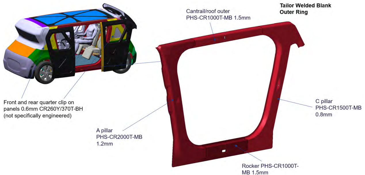
Figure 7.2.5.20 SEM1 outer ring and approach for A surfaces (See Appendix 4 for larger image)
