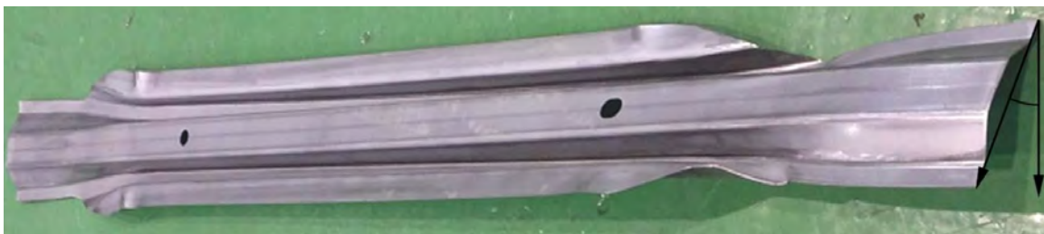
Figure 5.9: A roll stamped door part formed on a conventional roll forming line eliminates the need for welding brackets at the edges.
