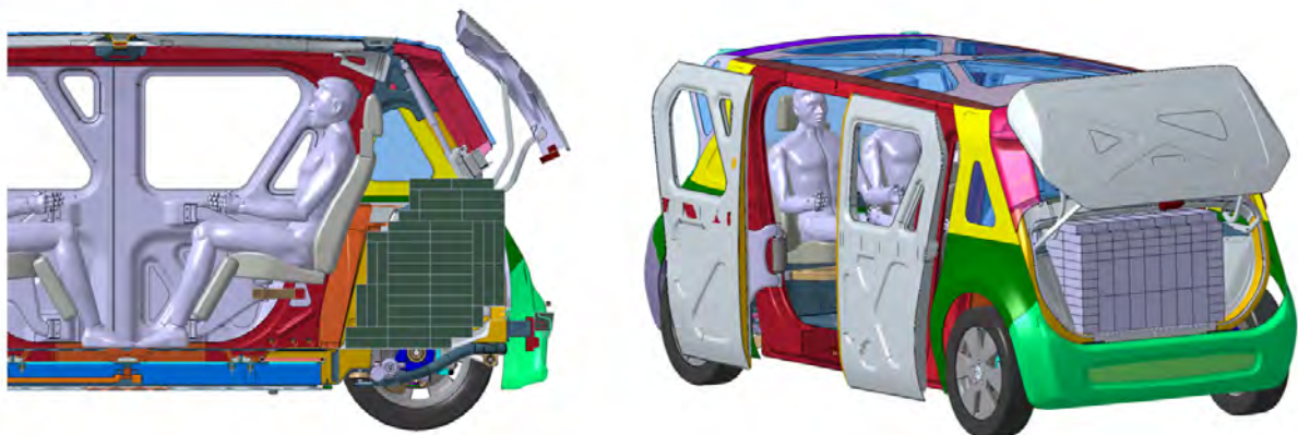
Figure 7.1.3.6 SEM1 luggage capacity estimation. 388litres
