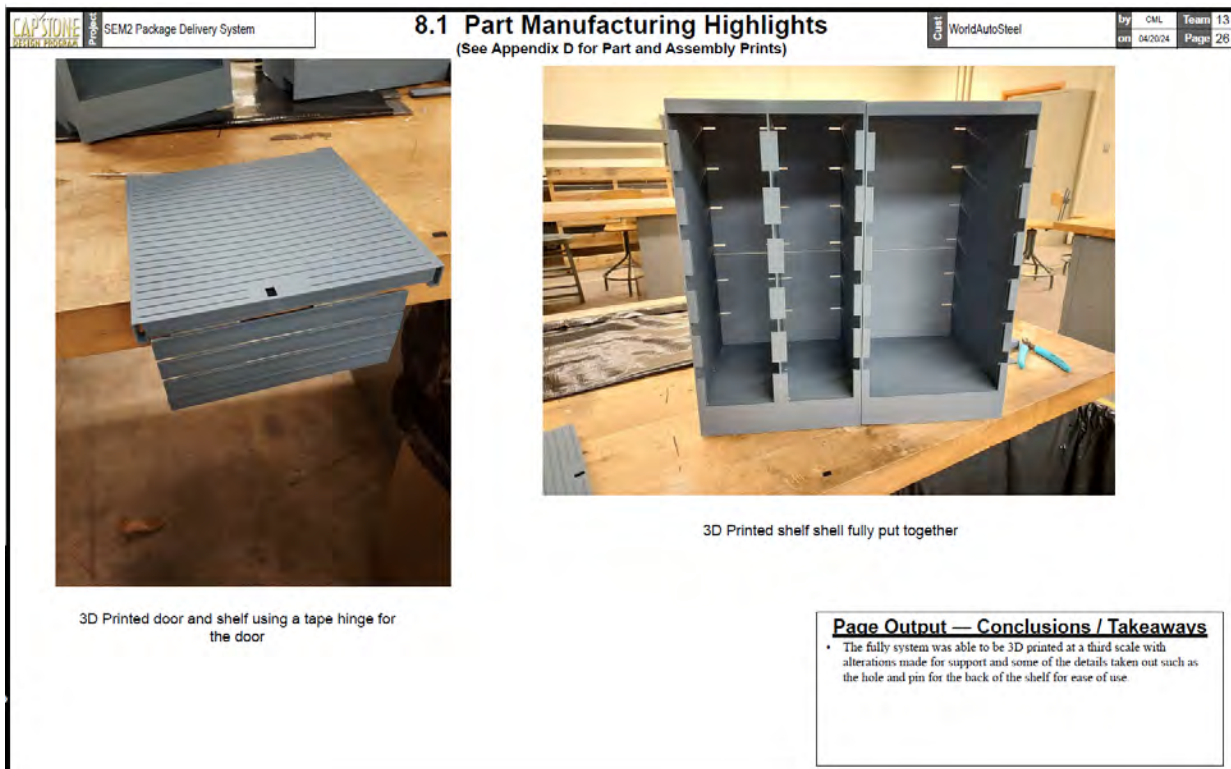
Figure 12.5.9 1/3 scale prototype model build of locker system.
