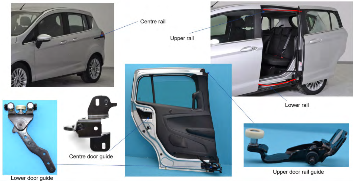
Figure 6.3.5.1.1 Track and rail sliding door, Ford B-Max passenger car (images from a2mac1)
