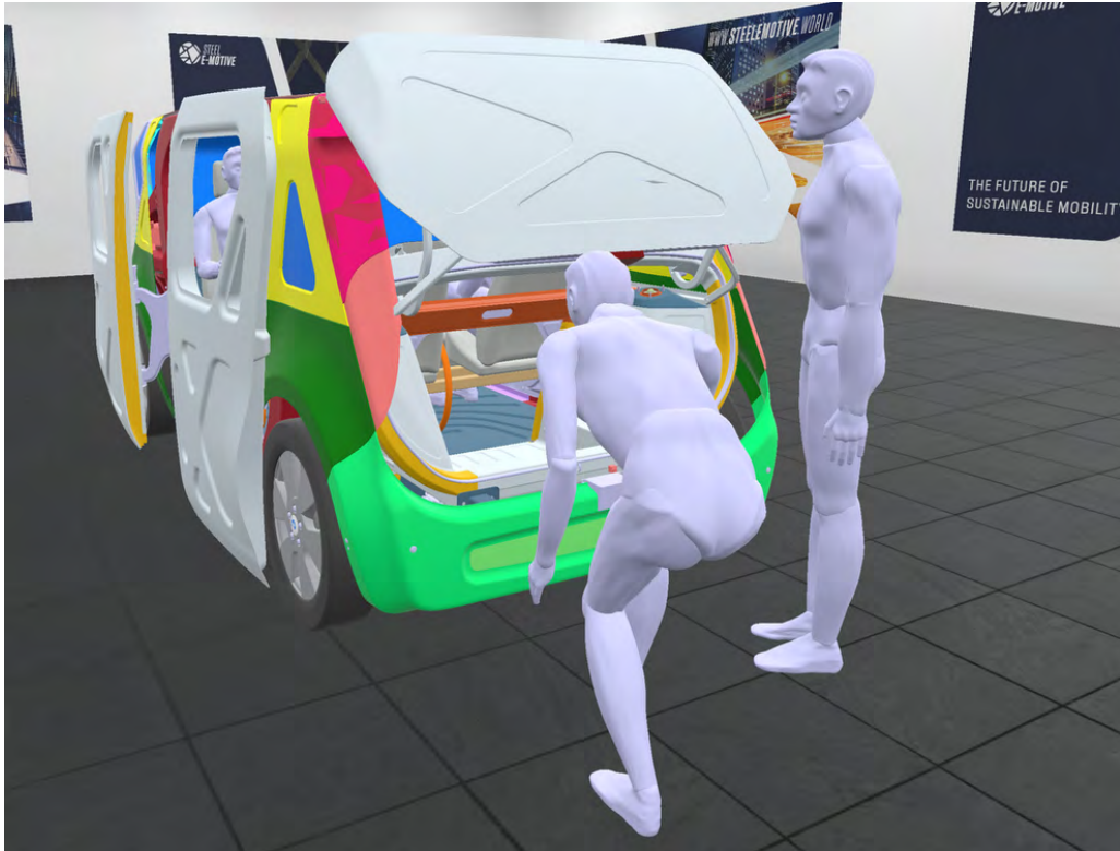
Figure 7.1.3.3 rear compartment access evaluation using Virtual Reality tools.
