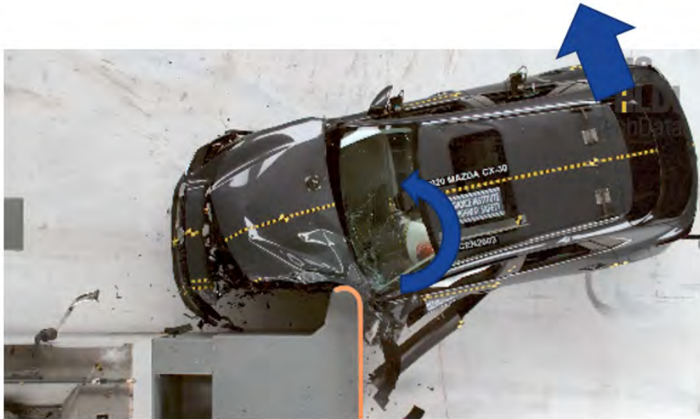
Figure 6.3.6.2.2 Mazda CX-30 2020MY, IIHS small overlap test
