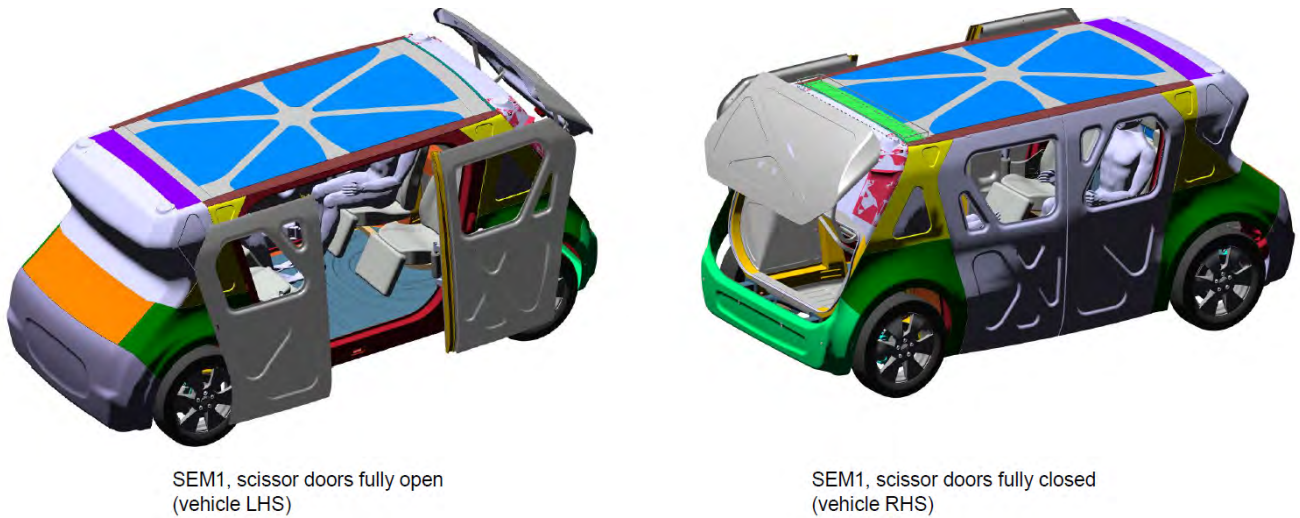
Figure 7.4.1.2.1 SEM1 scissor doors – open and closed positions
