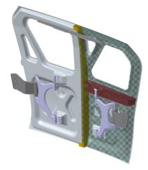
Caption: Scissor Door with Virtual B-Pillars creates a compact section for better passenger visibility. improving passenger access and enabling better side crash performance. Bake Hardenable steel's Class A-quality surface enables complete elimination of the body side outer for mass and cost savings.
